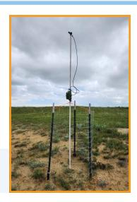
Acoustic detectors for bats will be set up within nearly every kilometer along the proposed route. Field technicians will assemble detectors (example shown here, although fencing around support stakes may not be required at every setup), and will leave them at the survey site for 4 to 7 days. Detectors may also be installed on fences. Field technicians will then return after the 4-7 days to retrieve the detectors.
